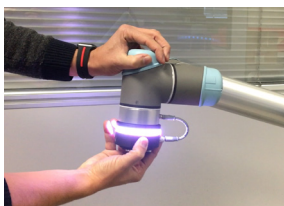
Enable the freedrive mode by clicking the black button
