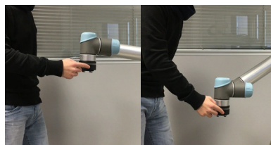
Save the current point by clicking the blue button
